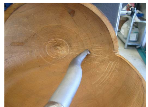
Cutter should always be on a 30 to 45 degree angle
